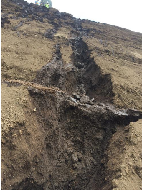
Figure 3. Damage caused by hydraulic energy. The image shows the hydraulic load and hydraulic gradient. At the top low hydraulic load is applied. Since the stream goes down the load increases. Kindly by Vetiver tec, Guatemala.
