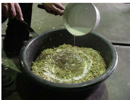
Figure 1 The Completed Mixing Adhesive was poured over Vetiver Grass Chips
