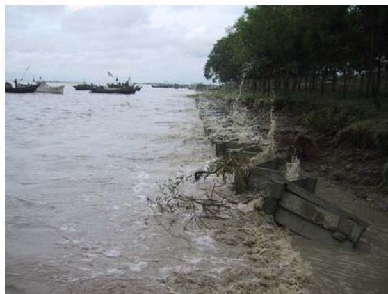
Fig. 8: Two months old Vetiver washed the highest tide of the year (August 08, 2002)
